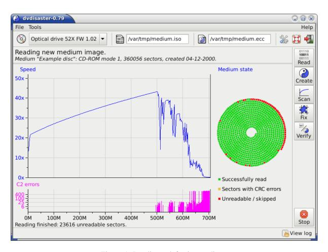
Figure 1: Reading a defective medium.
